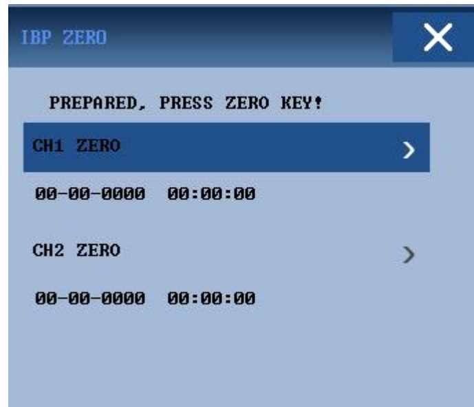
Figure 13-4 IBP Pressure Calibration
